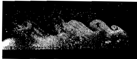
Figure 8.40 (a) and (b) Density currents observed in laboratory tanks. (From Simpson, 1969. Reprinted with permission from the Royal Meteorological Society.)
