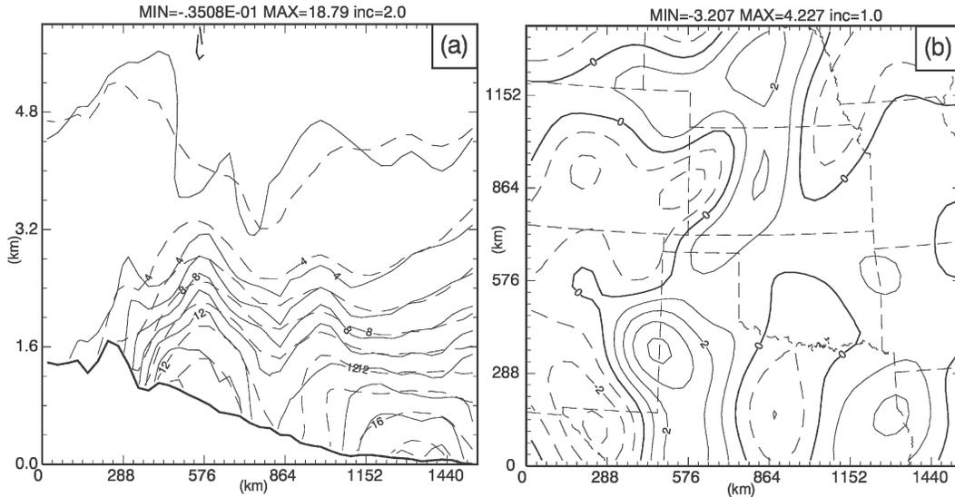
FIG. 7. (a) East-west vertical cross section of specific humidity field ( $\text{g kg}^{-1}$ ) at  $y = 234$  km where solid lines are for nature and dotted lines are for experiment SNF. (b) Analysis increment of specific humidity ( $\text{g kg}^{-1}$ ) at the surface from experiment SNF, where dashed lines are for negative values and solid lines are for positive values.
