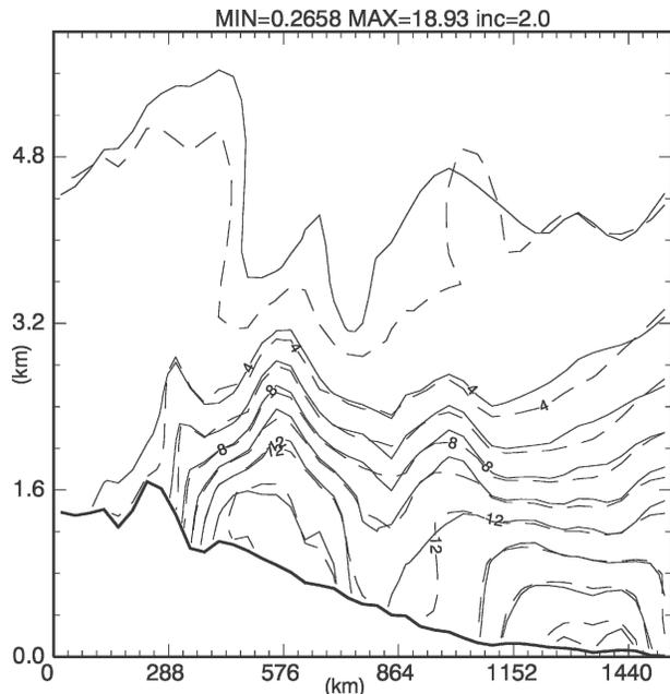
FIG. 5. East–west vertical cross section of specific humidity field ( $\text{g kg}^{-1}$ ) at  $y = 234$  km. The solid lines are for nature and the dotted lines are for CNTL.
