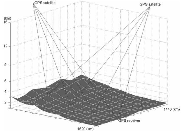
FIG. 2. A schematic of a ground-based GPS observation network whose data are analyzed using 3DVAR. Shaded surface represents terrain. Dark solid lines are slant paths between ground-based GPS receivers and GPS satellites. Dotted lines give a sense of the vertically stretched grid although the actual grid levels are in terrain-following coordinate.
