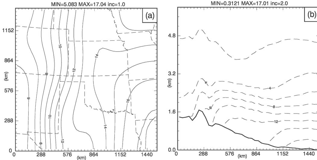
FIG. 4. Background specific humidity field in  $\text{g kg}^{-1}$ , obtained by smoothing the nature 50 times using a nine-point filter in the horizontal: (a) at the surface and (b) in the east–west vertical cross section at  $y = 234$  km.
